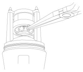
Remove the old cartridge by pulling off the rubber loops from the three shock-mount posts.
