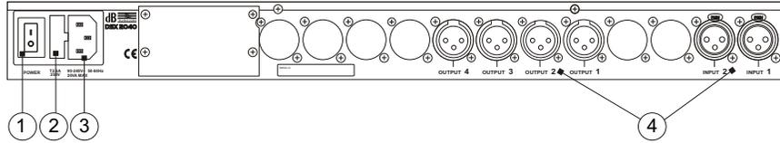
1. Main Power - Connects via a standard IEC socket. A compatible power cord is supplied with the unit. The voltage input is 90-240VAC, 50-60Hz.
